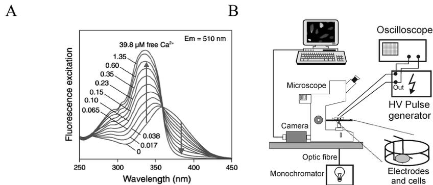
**Figure 1:** (A) Fluorescence excitation spectra of Fura-2 for different concentrations of Ca<sup>2+</sup> (image from <http://probes.invitrogen.com/handbook/figures/0554.html>). (B) Schematic of the experiment.
